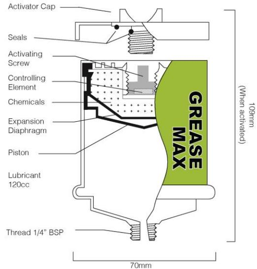
**GreaseMax** has no internal pressure prior to activation. Pressure is developed, and the lubricant discharge pressure is virtually in equilibrium with bearing or grease line resistance.
